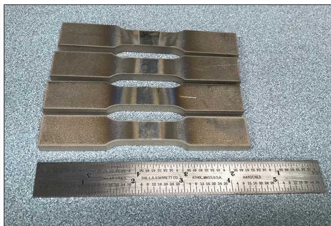
Fig. 2 — Final Nickel 201 samples used in SSR testing with the welded gauge section.
