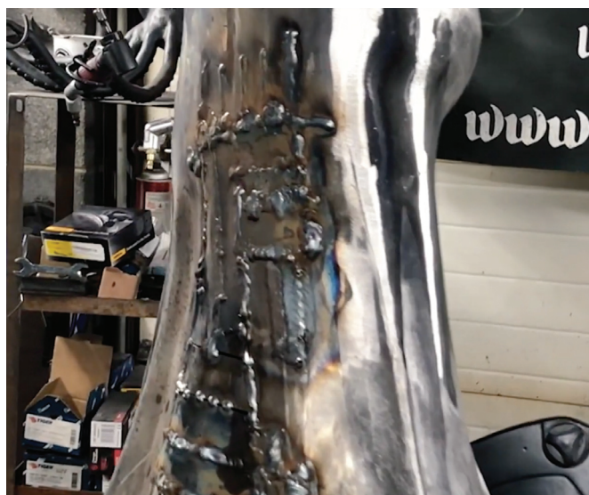
Fig. 2 — Welds from reshaping the statue's dress.
