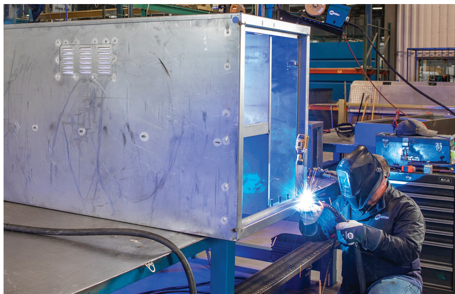
Fig. 8 — A welder performs gas metal arc welding in a manufacturing setting. This year accentuated some of the existing challenges in the welding industry, including labor issues, and the current environment further exposed the need for productivity-driven equipment solutions.
