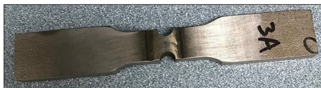
Fig. 6 — Final 52MSS sample with circular notches in the weld metal.
