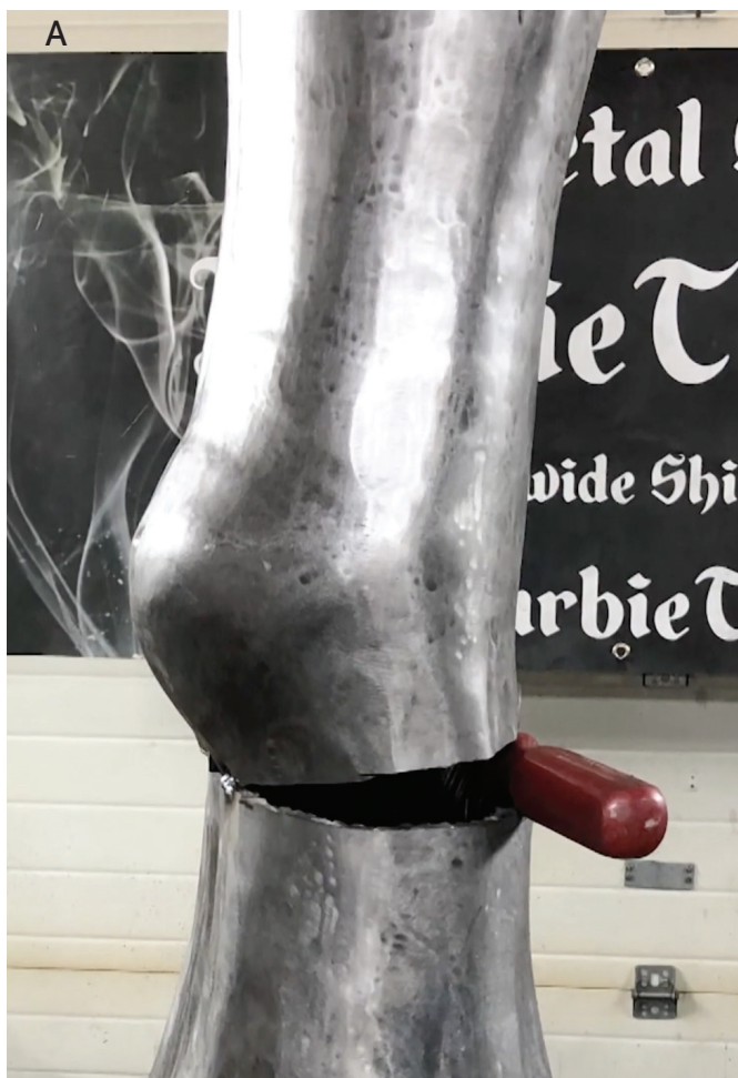
Fig. 2 — Welds from reshaping the statue's dress.
