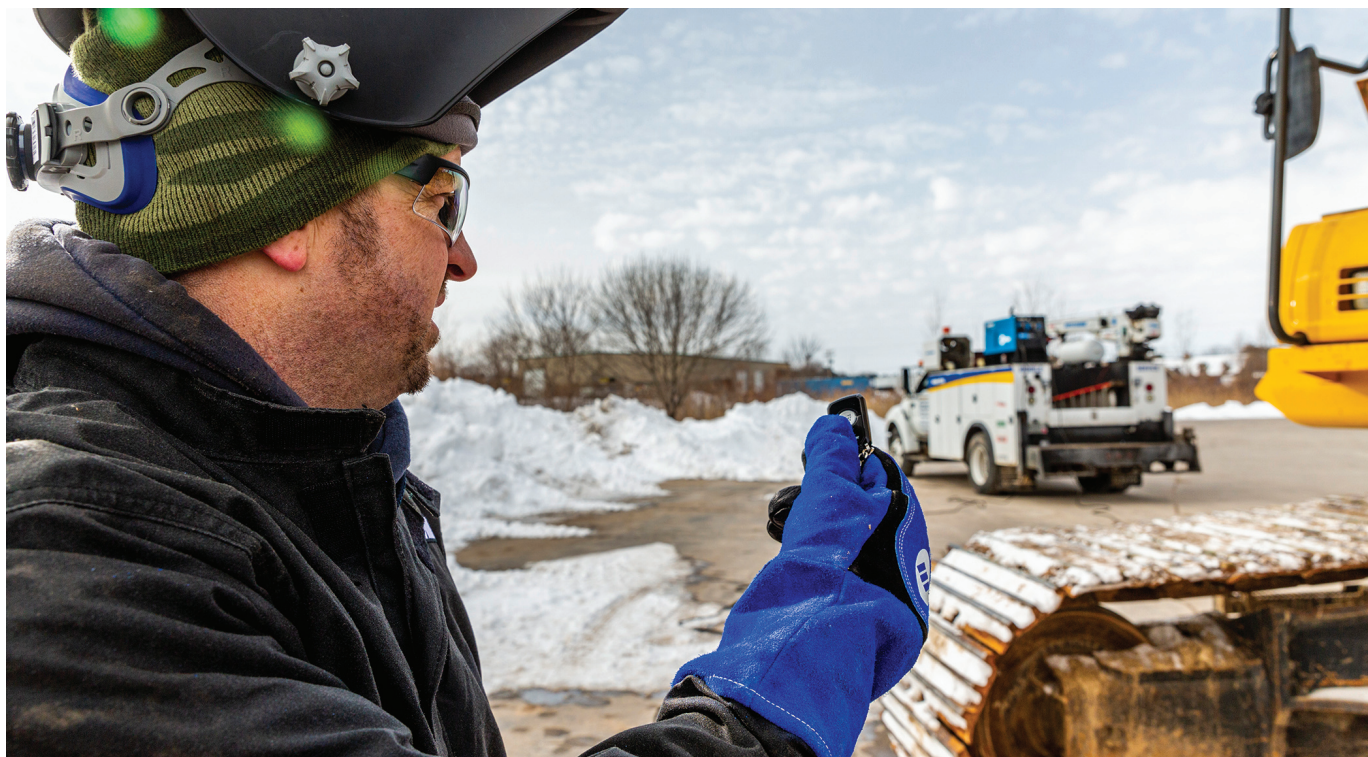
Fig. 2 — Remote start/stop on the Bobcat™ 260 and 225 lets operators easily turn the welding machine/generator on and off without having to walk back to the unit.
