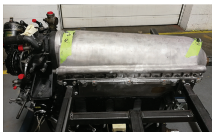
Fig. 6 — Gipsy DH Major 10MK1-3A engine assembled and readied for delivery.
