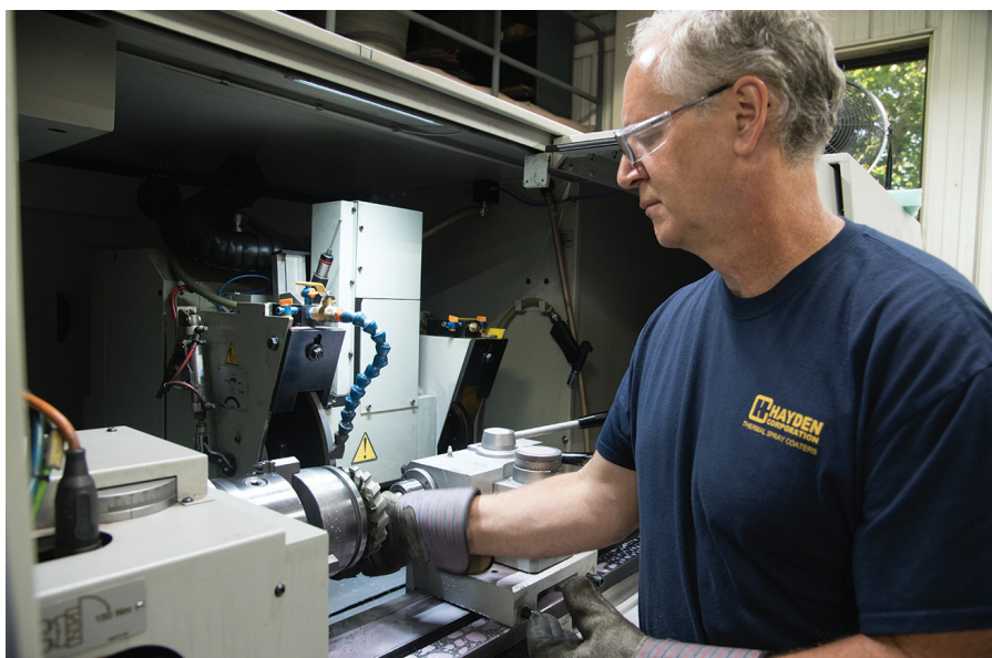
Fig. 5 — Tim Bernard works at a computer numerical control grinder.
